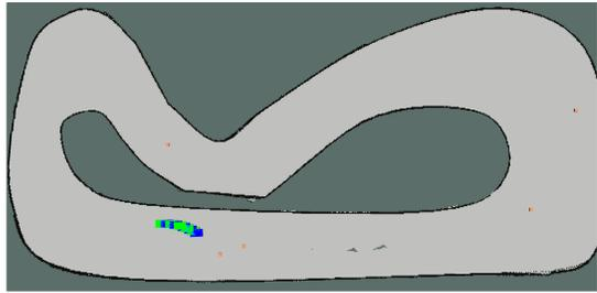
Fig. 1. Visualization of the set of reachable states using the current control action. For illustration purposes, we display only a subset of the hyper-rectangles (alternating green and blue boxes) making up the reachable set. This example corresponds to a safe scenario, as there is no intersection with obstacles or the racetrack walls (black). The orange squares represent the location of cones and their corresponding bounding box.
